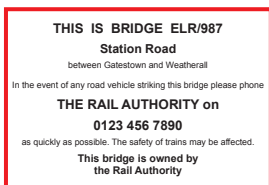
Example identification plate at a Network Rail bridge
