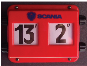
Notice in a driver's cab displaying the overall vehicle height
