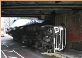
A curtain sided lorry overturned as a result of a bridge strike
